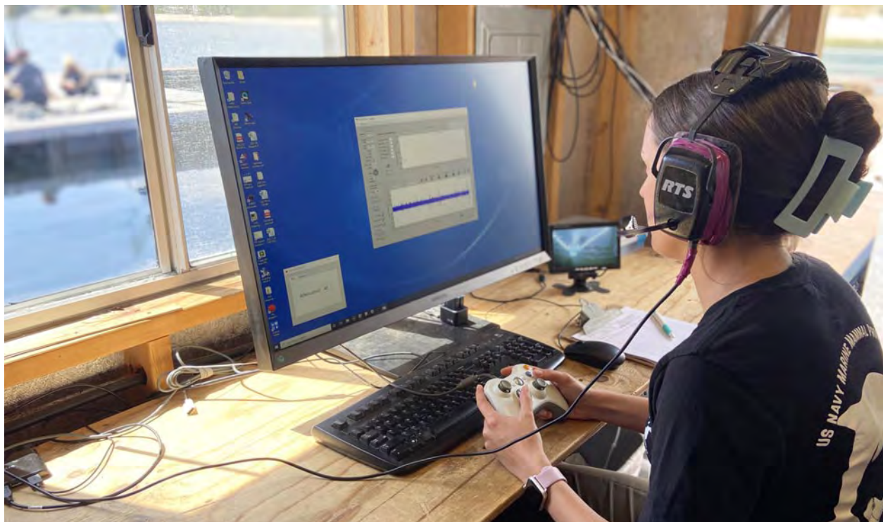
The hearing tests are conducted from an experimental shack located near the dolphin's floating netted enclosures. Researchers communicate with trainers via headset and monitor the dolphin's behavior using a listening hydrophone and video camera.
