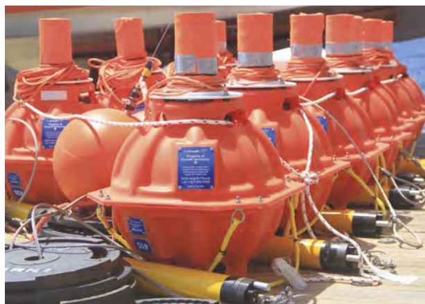
Rockhopper acoustic recording devices ready for a research deployment.
